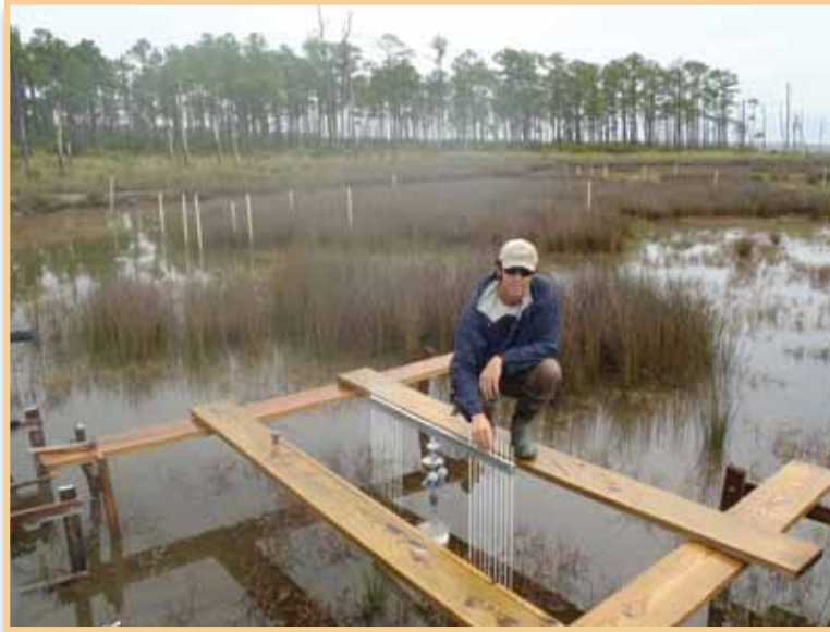
Figure 20. Measuring accretion at surface elevation tables.
