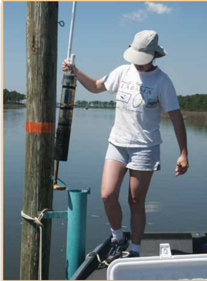
Figure 18. Rotating data sondes at Grand Bay NERR SWMP station.
